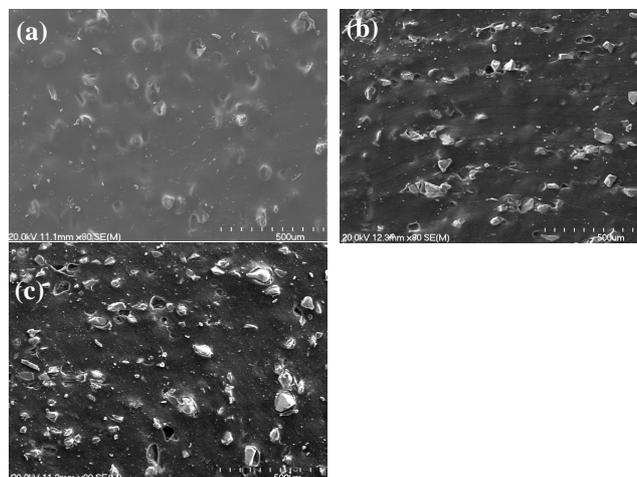
Figure 1: SEM images of MREs (a) isotropic, (b) anisotropic and (c) anisotropic with carbon black reinforcement
